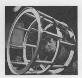
FINISHED FABRICATION JOB of welded aluminum pieces is examined by Charlie Bates. The precision job is typical of the majority of the work performed by men of the Sandia Laboratory's Welding Shops.
